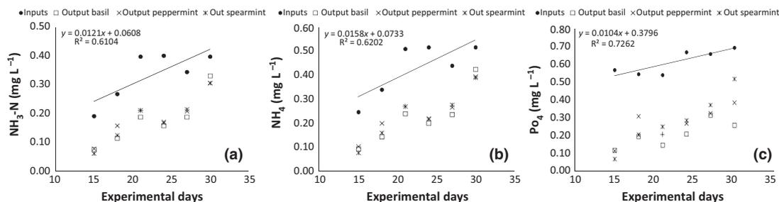
**Figure 2** Metabolites concentration in water ( $\text{mg L}^{-1}$ ) inputs and outputs of biological filters according to the herb species used, for tilapia culture in aquaponics systems. (a) Un-ionized ammonia ( $\text{NH}_3\text{-N}$ ), (b) Ammonium ( $\text{NH}_4$ ) and (c) Phosphates ( $\text{PO}_4$ ).
