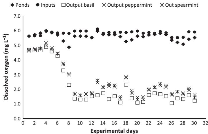
**Figure 5** Dissolved oxygen values (mg L<sup>-1</sup>) in ponds, inputs (*n* = 9) and outputs (*n* = 3) from hydroponic beds according to the herb used as part of biological filter for tilapia culture in aquaponics systems, along experimental period.
