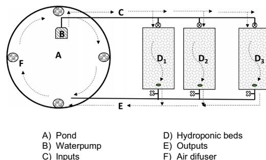
**Figure 1** Items in the aquaponic system used. Not to scale.
