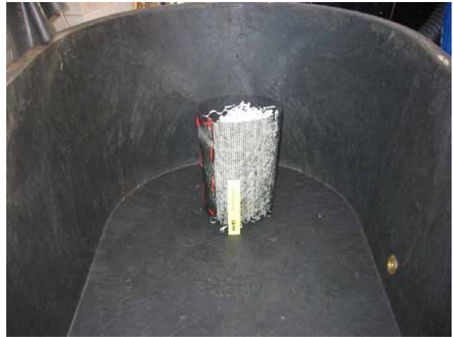
9. A cattle watering pan with a biofilter that will be submerged; a 6-inch ruler is shown for size reference.
