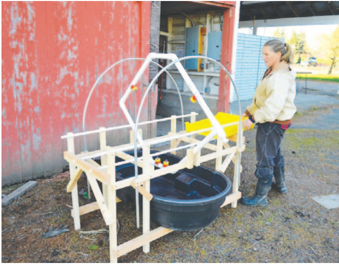
This is how bins slide through the washer. When in use, a tarp is put over the hoops to keep water from going everywhere.
