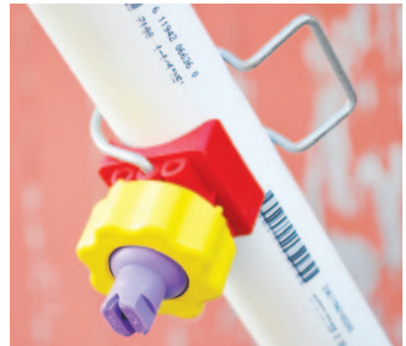
At left is the author's adjustable-height rolling table, with storage shelves over and under the table surface. Above are K-Ball nozzles used in the tote washer on the facing page. They can turn a piece of PVC pipe into a section of sprayer simply by drilling a hole in the pipes and clipping on a nozzle, available from US Plastic Corp.
