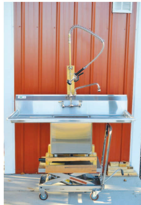
The author's adjustable-height washing sink, with detail showing the stainless steel grate that can be added to use it as a spray table.
