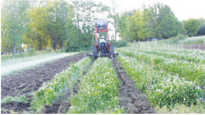
Loosening soil before planting in fall-tilled strips with a two-shank subsoiler. Compost tea flows from the tank on the tractor bucket to the subsoiler shanks, applying compost tea every four inches, down to a depth of 16 inches, along the shanks.
